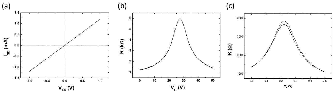
(a) Output curve, measured at room temperature and vacuum conditions. (b) Transfer curve under back gating measured at source-drain voltage of 20mV, under same conditions as (a). (c) Transfer curve under liquid gating through Phosphate Buffered Saline (PBS, pH=7.3), using the on-chip electrode as gate electrode.
